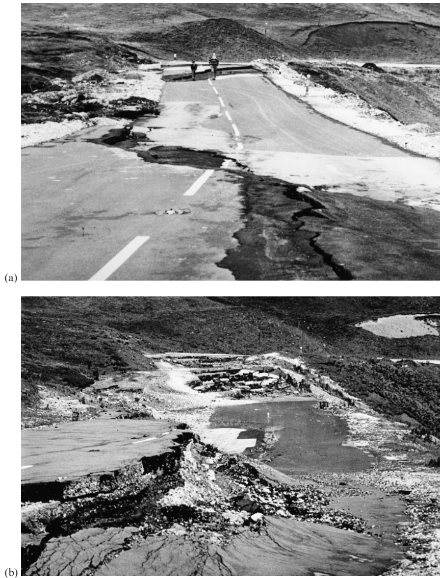
Fig. 17. Displacement of the upper road where it crosses landslide element M. Photographs were taken in (a) 1977 and (b) 1998. Movement is downwards and to the right at a mean rate of 0.25 m per year.
